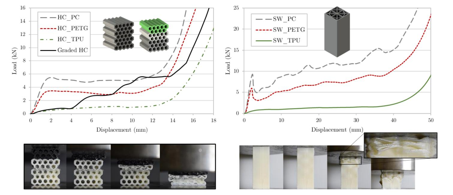
Figure 5 – Collapse behaviour of multi-material (left) and single material developed EAS
