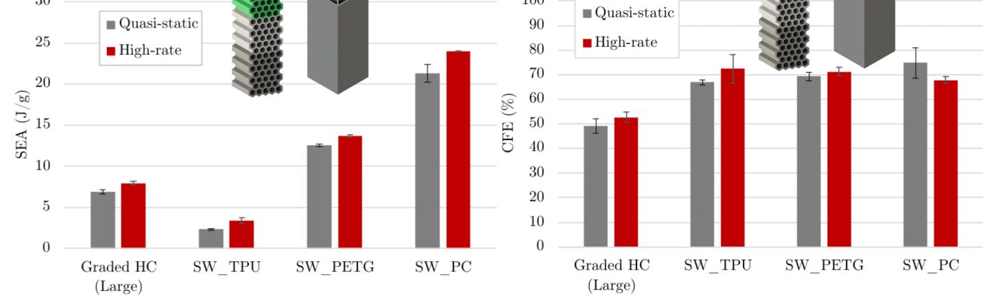
Figure 7 – Calculated SEA and CFE values for multi-material honeycomb and spider web graded structure, under quasi-static and high-rate compression.
